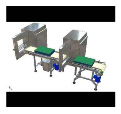
Machine design criterion: The conveyors are designed to transport cartons to and from a strapping machine
